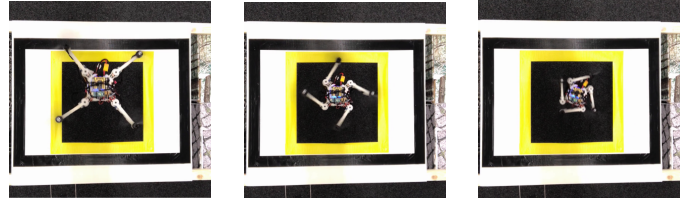
Fig. 6: Traversal of an horizontal gap using the O morphology. Left: the quadrotor approaches the gap with the X configuration (time t = 0 s). Center: the quadrotor starts the folding maneuver to adapt its morphology to the shape of the gap ( t = 1 s). Right: the gap has been traversed ( t = 2 s).
